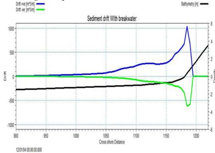
Fig.4: Graph for littoral Drift with Breakwater.
