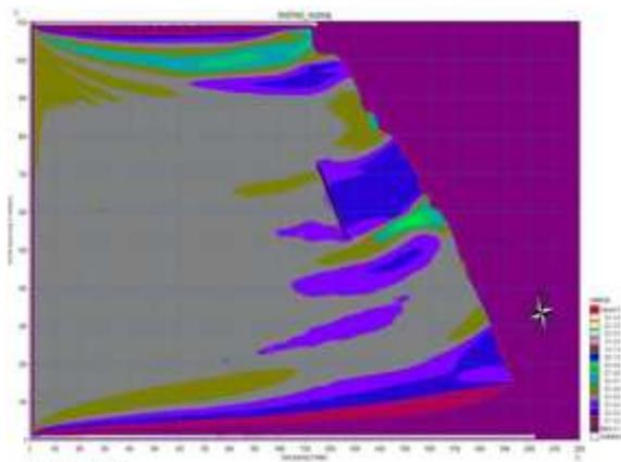
**Fig. 8:** Significant wave height with permeable breakwater (WEC) with angle of wave incidence 280°
