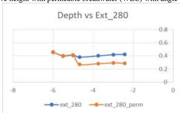
**Fig2:** Graph between water depth Vs significant wave height for angle 280°, without the permeable breakwater (WEC) and with the permeable breakwater (WEC).
