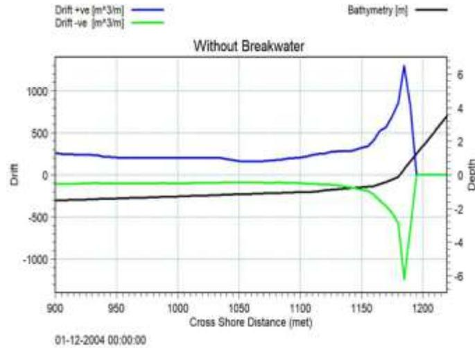
Fig.3: Graph for littoral Drift without breakwater
