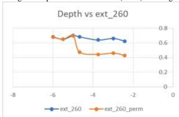
**Fig.1:** Graph between water depth Vs significant wave height for angle 260°, without the permeable breakwater (WEC) and with the permeable breakwater (WEC).
